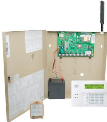
NuMed will incorporate a commercial standard alarm control panel. The alarm panel provides multiple zones of protection, an always-on Department IP connection, graphic keypad support and dual partitions. The alarm panel provides the ability to send alarm signals and upload/download via an Internet Protocol. The control panel will send a signal or polling to the alarm company every 200 seconds to ensure the system is in good working order and transmitting to the alarm company.
